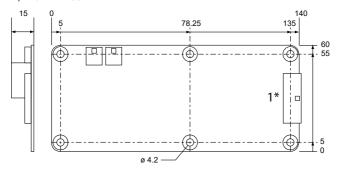
1\* is 1 mm longer than the PCB dimensions 10 mm copper circumferential on the rear side 8.4mm on the front side Dimensions in mm
