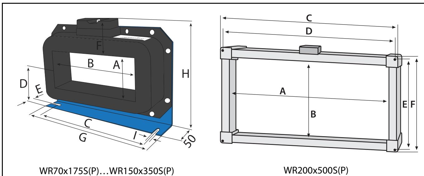
**Abmessungen (mm), Gewichte (g)****Dimensions (mm), weight (g)**
