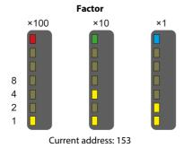
Addresses can only be entered within the valid address range. When there is no input for a period of 5 minutes, the device automatically exits the address setting mode. The device then uses the currently set RS-485 address.
