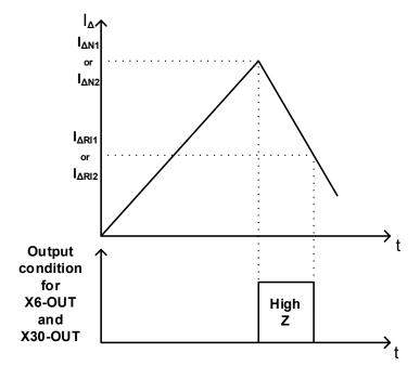
Fig. 1: Meaning of switching recovery level
