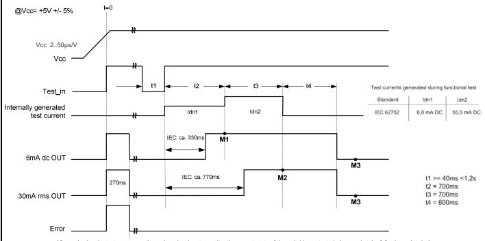
After activating the test sequence, the end product has to monitor the correct state of the switching outputs being used at the following points in time
