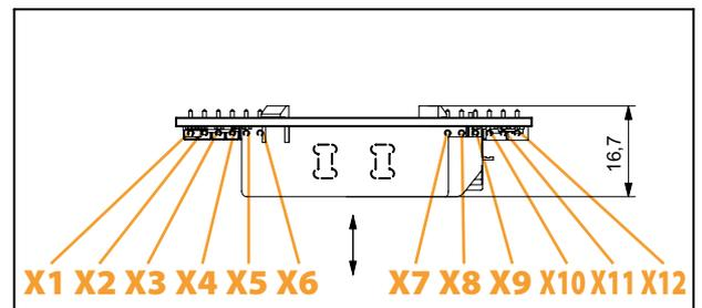
**Base plate of 1.7 mm thickness, tolerance: + 0.1 mm/- 0 mm**
